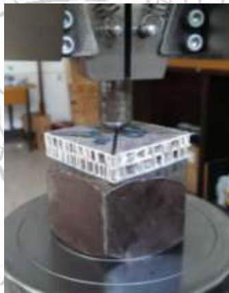
Fig. 4. Multilayered honeycomb composite material in test position
