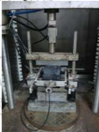
Fig. 5. Apparatus for determining the stiffness module
