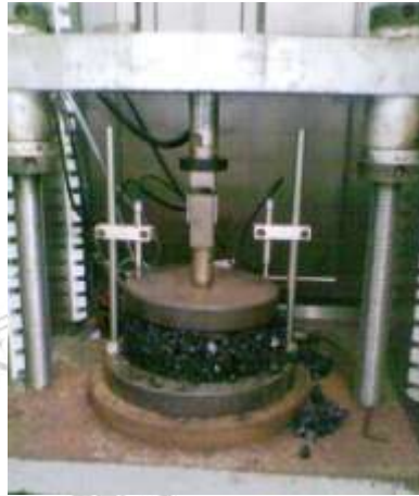
Fig. 4. Cyclic compression test apparatus (Dynamic Variation)
