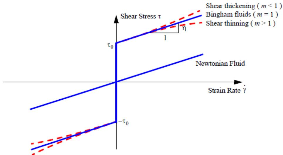
Fig. 6: Visco-plasticity models of MR fluids
