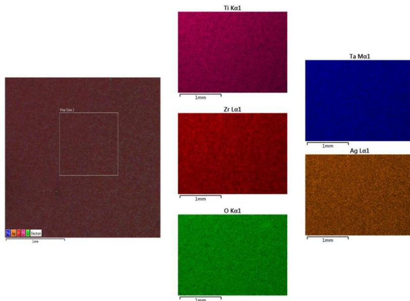
**Fig. 1.** Surface mapping of alloy V1 by EDX
