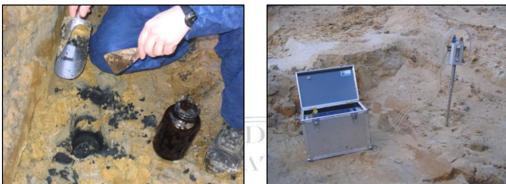
Fig. 3. Soil and soil gas sampling at the former fuel station.
