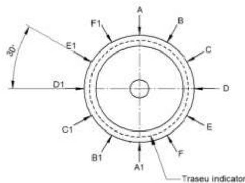
**Fig. 7.** Measurement scheme of circularity.
