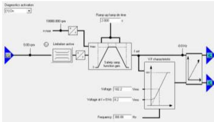
**Fig. 3.** Setting the time of acceleration / deceleration.
