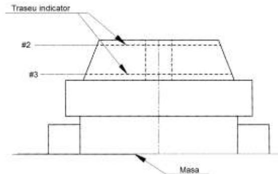
**Fig. 8.** Verification scheme of the tilt angle.
