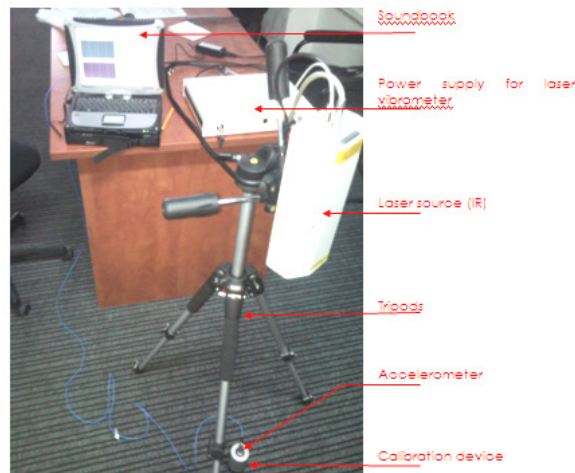
Fig. 7. Installation with accelerometer and vibrometer
