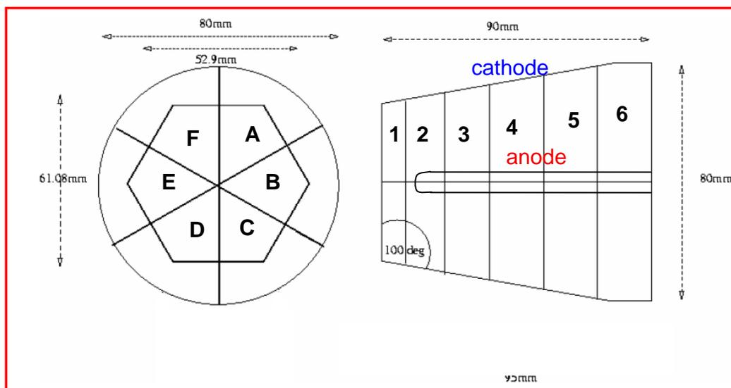
**Figure 3** The segmentation of a typical AGATA detector [4].
