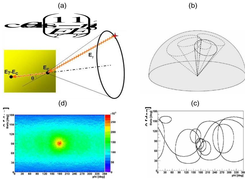
**Figure 5** Principle of the  $\gamma$ -ray imaging with a segmented Ge detector.
