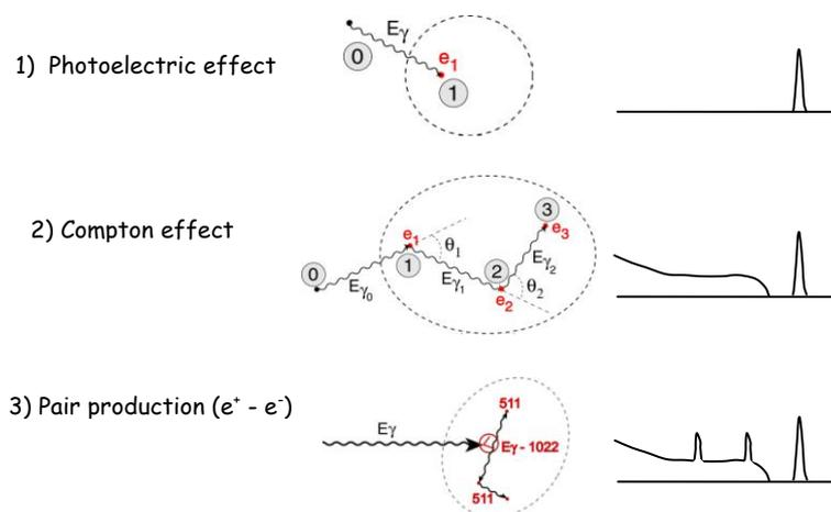
**Figure 1** Processes by which a gamma-ray (photon) interacts with a Ge detector; the left side shows the corresponding response (energy spectrum).
