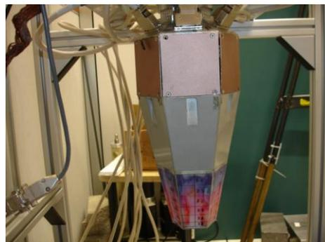
**Figure 6** Experimental arrangement for  $\gamma$ -ray imaging with an AGATA detector [6].
