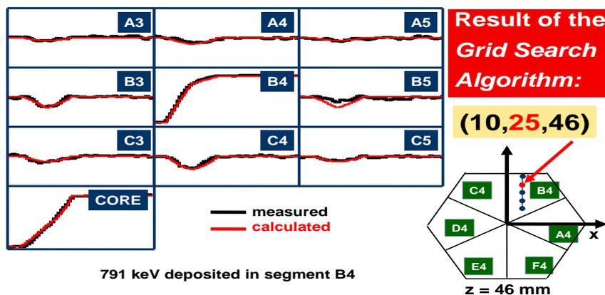
**Figure 4** Example of pulse-shape analysis of an interaction in an AGATA detector. A photon left 791 keV in segment B4, and the pulses given by this segment and its neighbors (see Fig. 3) are shown. The continuous lines are calculated with the specified algorithm, for different interaction positions. The best fit is obtained for the position  $(x,y,z) = (10,25,46)$  (relative coordinates in mm); calculations with  $y=20$  or  $30$  mm give much worse fits (ref. [6]).
