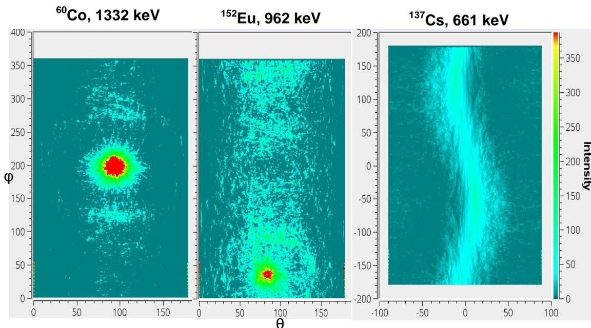
**Figure 7** Images of the three sources placed around an AGATA detector as shown in Fig. 6. The images shown here were obtained by tracking on the radiations with the indicated energies [6].
