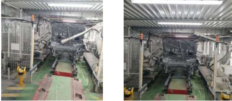
Fig. 5. Robots applying mastic cords in the engine compartment area. a. Robot at work; b. Robot at rest.
