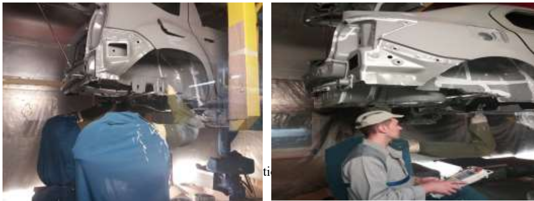
Fig. 15. Applying mastic under the bodywork.
