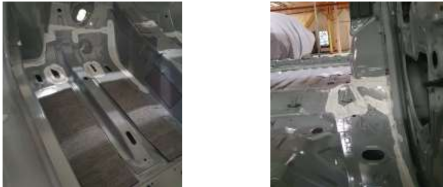
Fig. 3. Mastic cords applied in a manual process.
