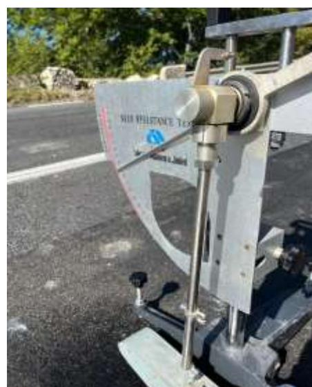
Fig. 8 Determination of roughness with the SRT pendulum
