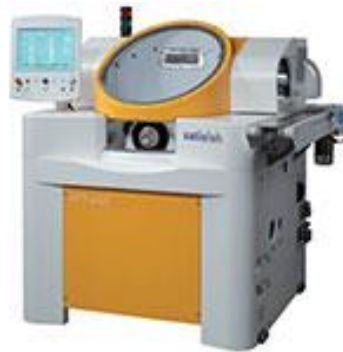
Fig. 2. Diopter generator - VFT orbit machine.
