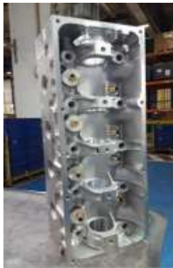
Fig. 1: K7 Cylinder head [1]
