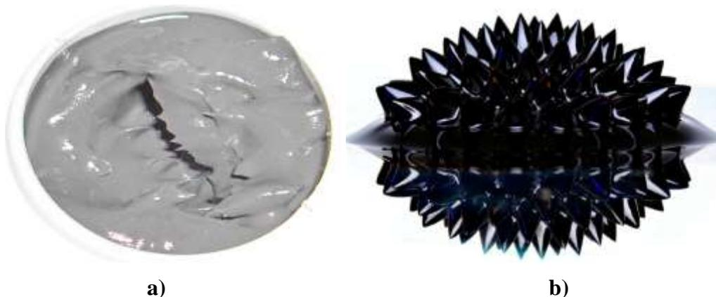
**Fig. 2:** Magneto rheological fluid (a) from Lord Corp. and ferrofluid (b), produced by Apexmagnets LLC.
