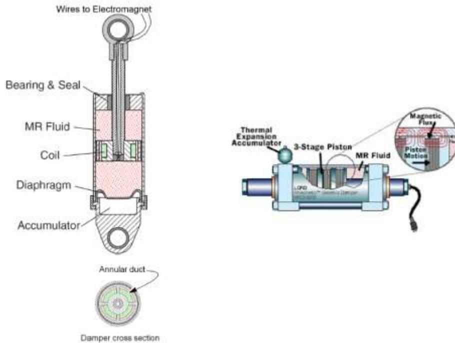
**Fig. 4:** Schematic of single ended MR damper and double ended MR damper, both produced by Lord Corp.
