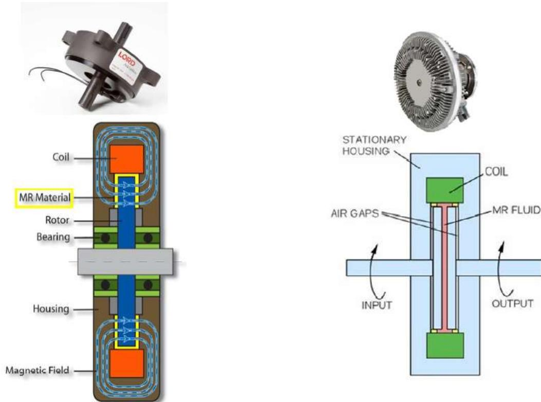
**Fig. 5:** Picture and schematic of MR based brake and clutch, both produced by Lord Corp.
