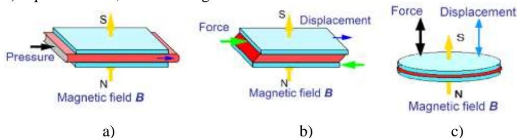
**Fig. 3:** Typical utilisation modes for MR fluids, flow (a), shear (b) and squeeze (c) mode.
