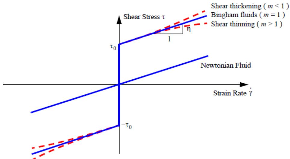
Fig. 6: Visco-plasticity models of MR fluids
