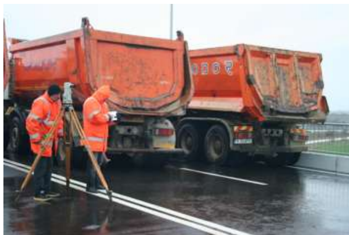
Fig. 6: Image from the levelling measurements [2]
