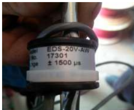
Fig. 9: Tensiometric transducer with rope [2]
