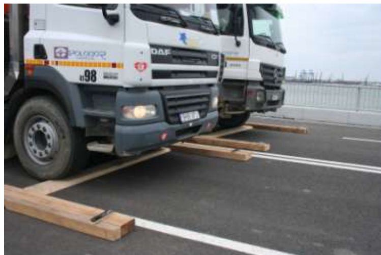
Fig. 12: Detail when passing the truck over the wooden threshold
