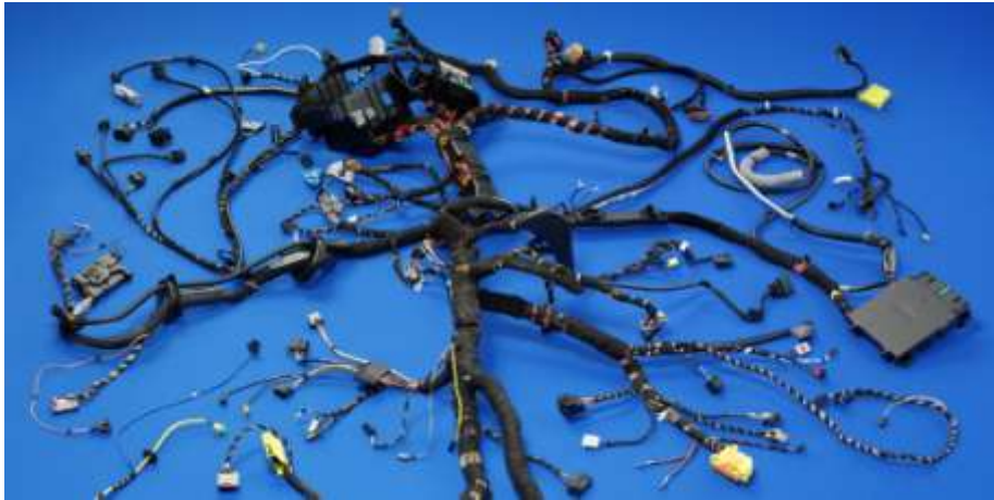
Fig. 2: Unassembled vehicle cable harness [6]
