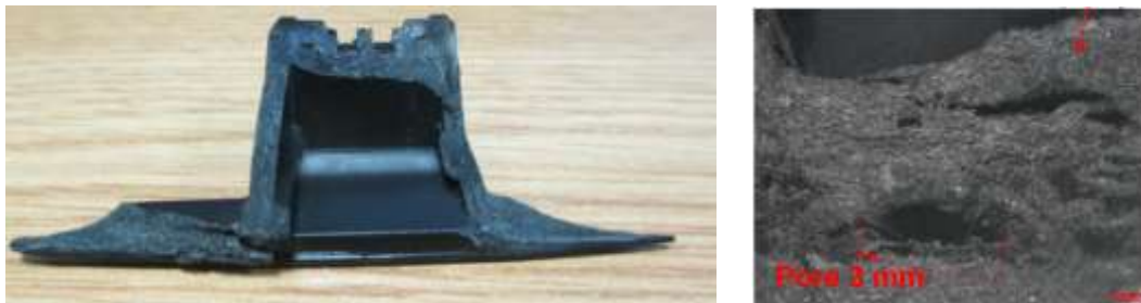
Fig. 6: Air gap defects in the rupture area
