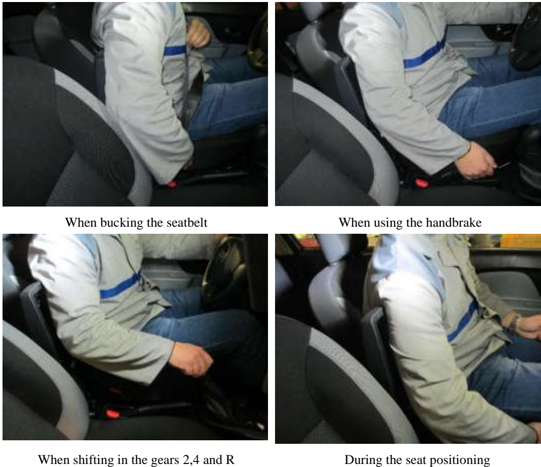
Fig. 8: Conditions when the armrest can be accidentally broken
