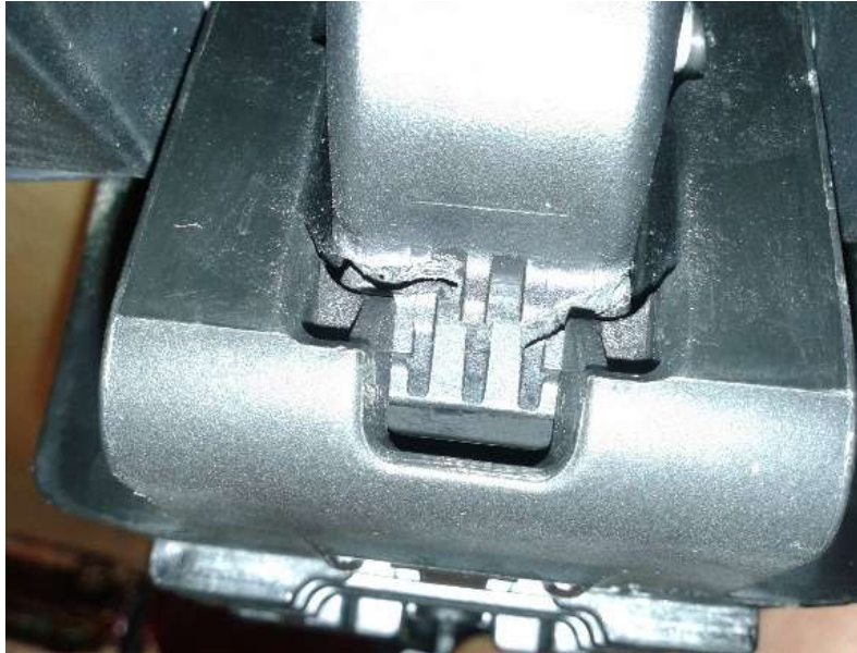
Fig. 2: Part breaking area
