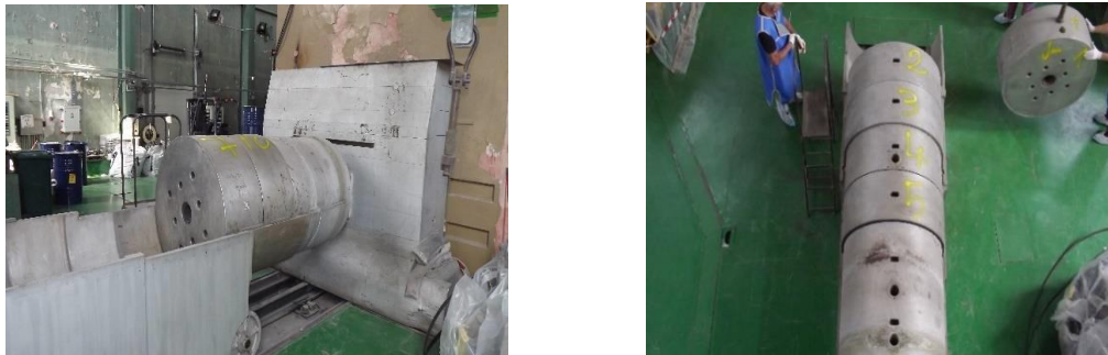
Fig. 1. Overview of the thermal column and its composing discs [1]
