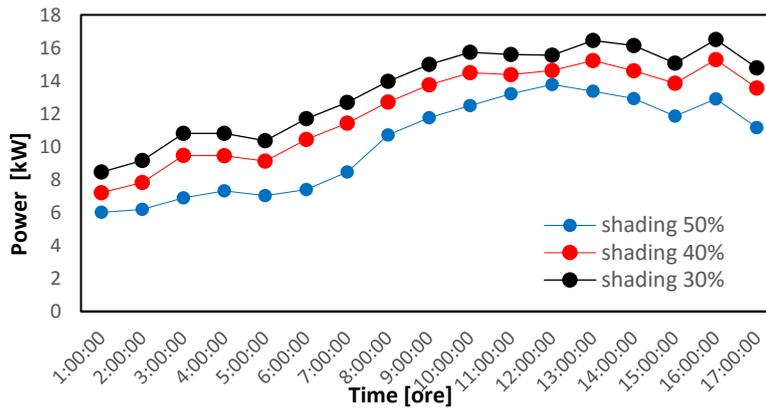
Fig. 4.1 PV generator behavior for different degrees of shading, conventional approach
