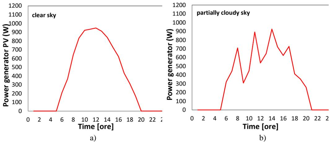
**Fig. 3.11** The daily evolution of power for the photovoltaic generator
