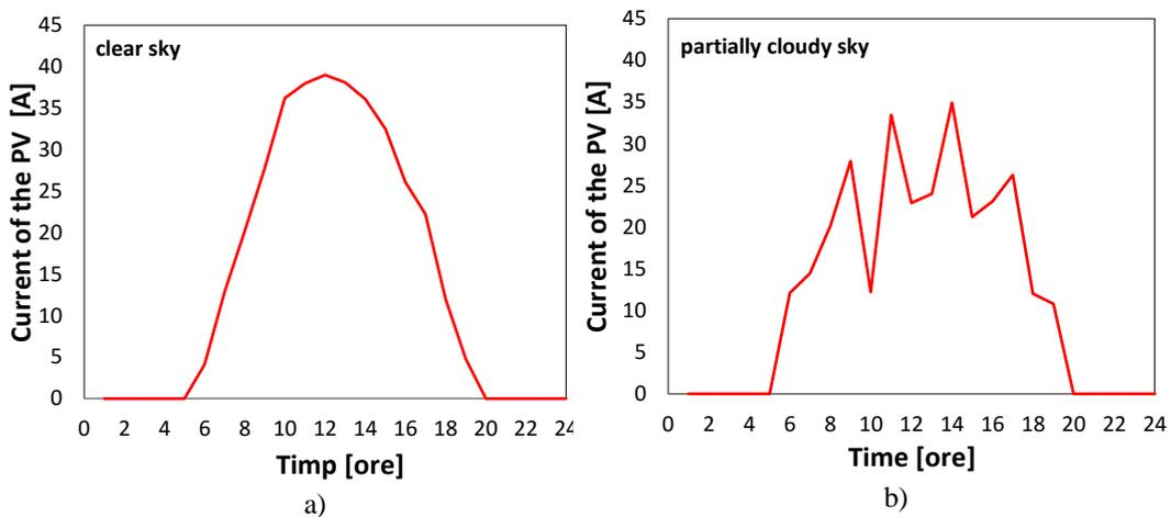
*Fig. 3.8 The daily evolution of the current for photovoltaic generator*
