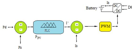
Fig. 3.15 Battery control units
