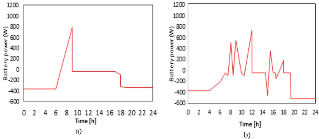
*Fig. 3.12 The daily evolution of battery power for the photovoltaic system*
