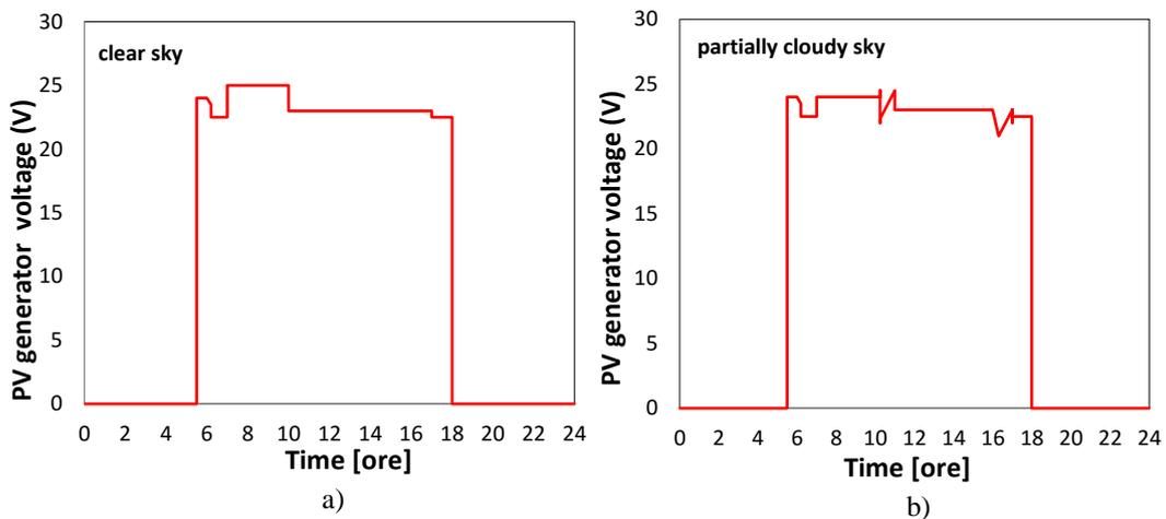
*Fig. 3.9 The daily evolution of the voltage for the photovoltaic generator*
