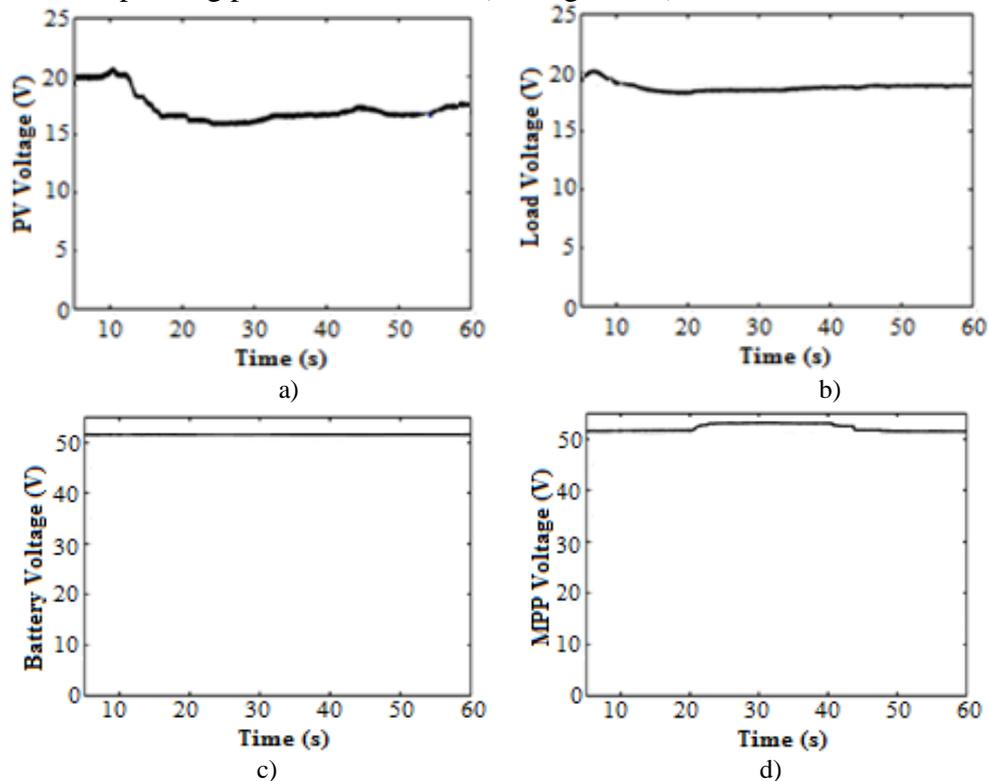
*Fig. 3.17. Voltage response in complex PV system. a) PV generator voltage; b) load voltage; c) battery voltage; d) MPPT voltage*
