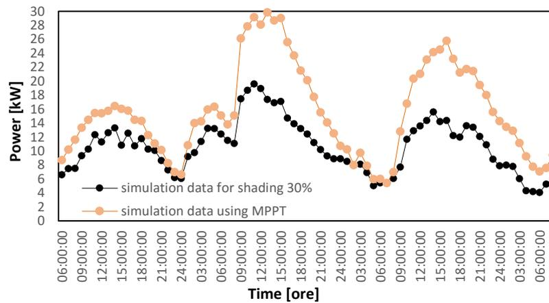
Fig. 4.4 The power generated by BIPV for 30% shading, MPPT approach
