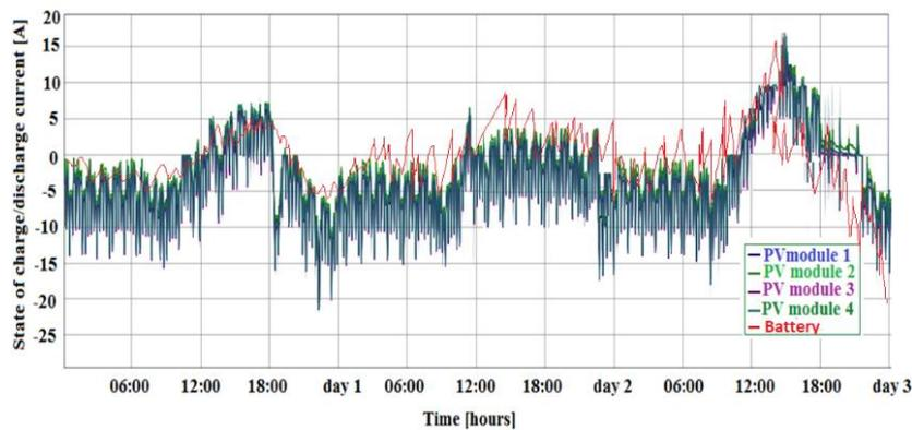
Fig. 3.19 System charging / discharging state (PV generator + electrical storage system)
