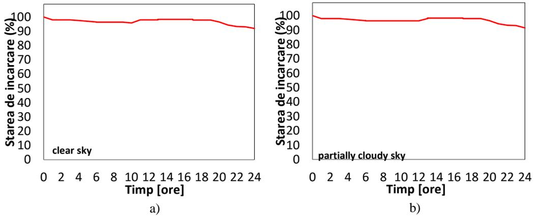
Fig. 3.6 (a & b): Battery charging state of the stand-alone photovoltaic system based on controller monitoring
