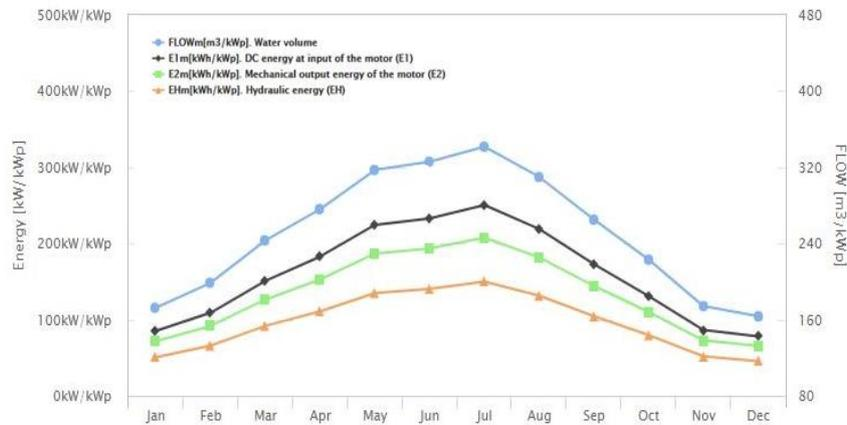
**Fig. 4.6** Overall performance of the PV pumping system
