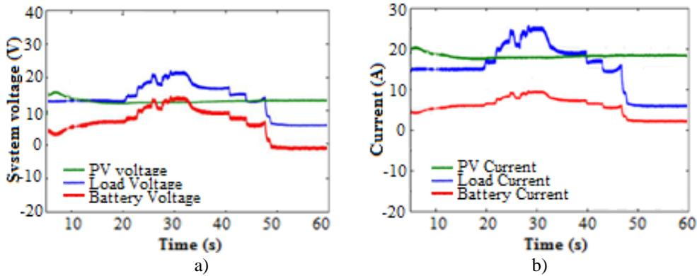
Fig. 3.18 Current and voltage behavior over time for different input and output parameters of the photovoltaic system (solar irradiation, load, battery voltage)
