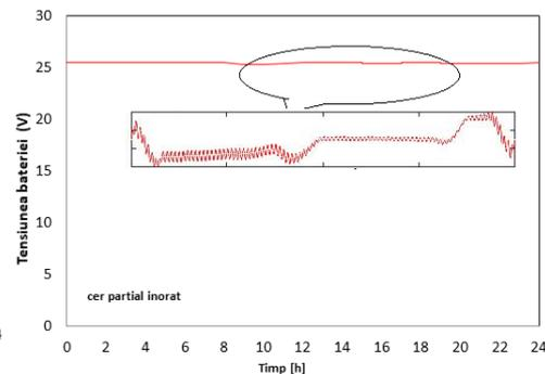
*Fig. 3.5 Behavior of battery voltage during a cloudy day*
