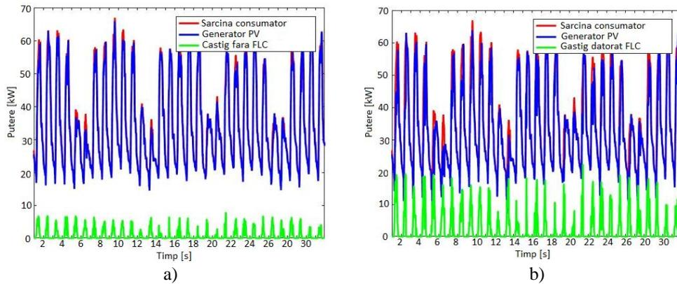
Fig. 3.22 System power gain recorded a) with no FLC and b) with FLC
