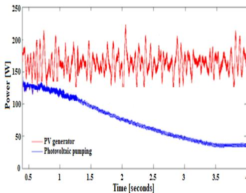
**Fig. 4.7** Performance of the PV pump with MPPT disabled
