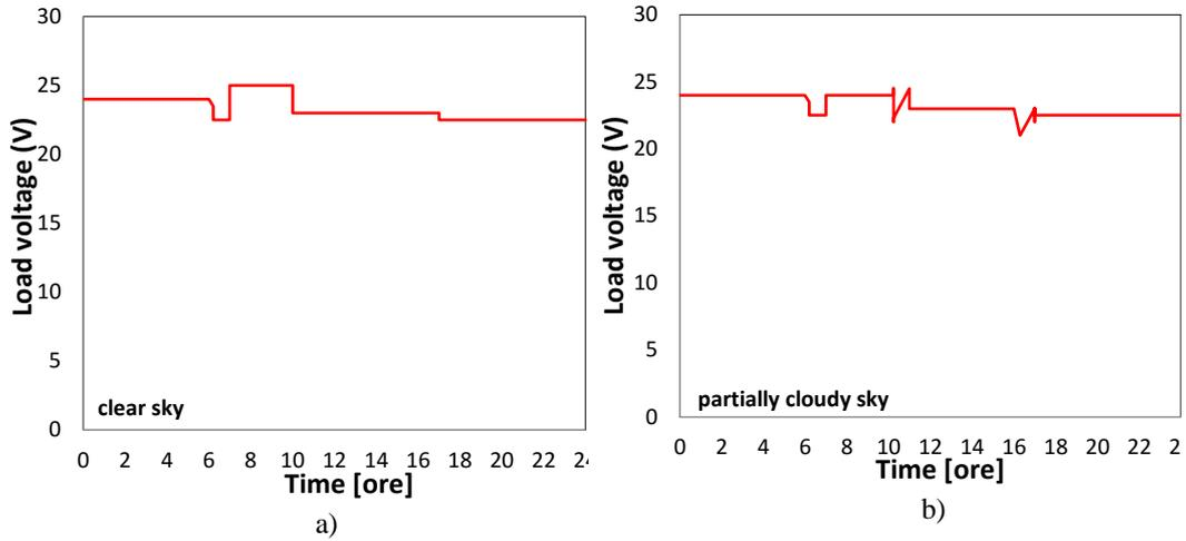
**Fig. 3.10** The daily evolution of the charge voltage for the photovoltaic system
