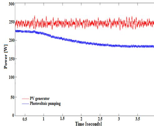
**Fig. 4.8** Performance of the PV pump with MPPT activated
