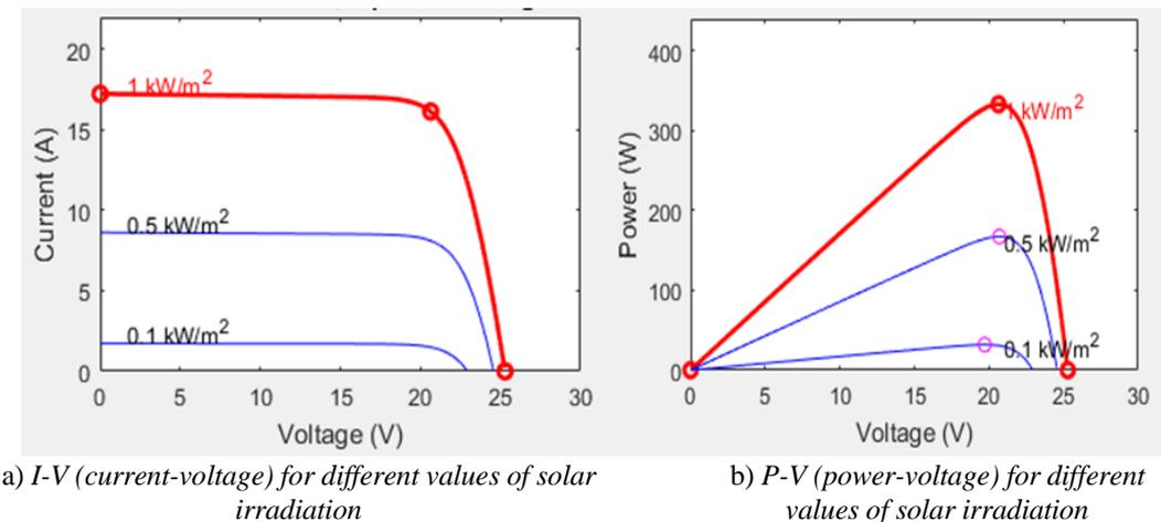
**Fig. 3.2** *I-V (current-voltage) and P-V (power-voltage) in the analysis of the PV generator for different values of solar irradiation*
