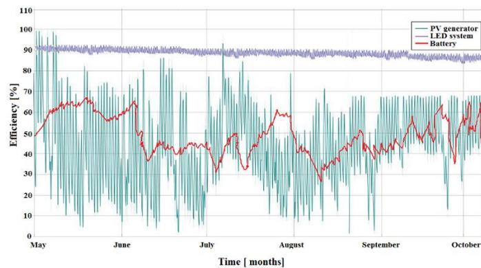
*Fig. 3.21. The long-term efficiency of the complex PV system*
