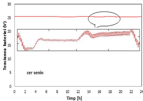
*Fig. 3.4 Behavior of battery voltage during a clear day*
