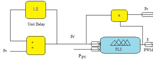
Fig. 3.14 MPPT Configuration of the MPPT - FLC controller
