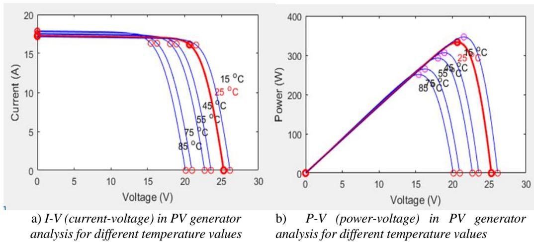
**Fig. 3.1:** *I-V (current-voltage) and P-V (power-voltage) in PV generator analysis for different temperature values*
