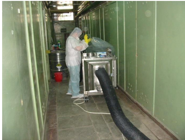
Fig. 3. Industrial vacuum machine fitted with HEPA filtration
