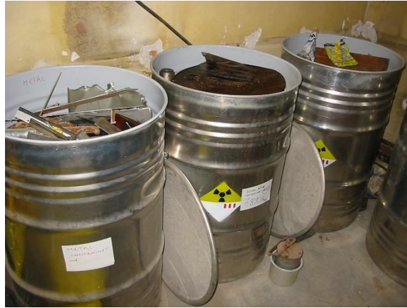
Fig.5. Containers with very low-level radioactive wastes
