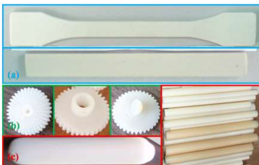
Fig. 1. (a) PA6 test samples processed by extrusion/ injection (same procedure used for finite products used directly into industry) that were subjected to recycling process, (b, c) example of finite products (gears, bars) made from PA6 manufactured through extrusion/injection
