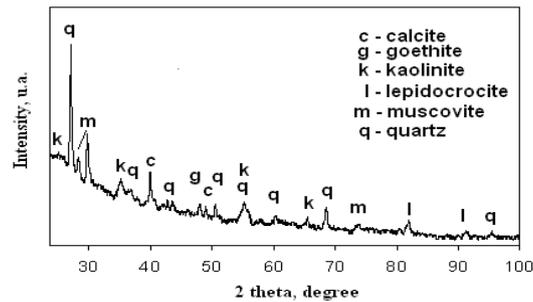
**Fig. 8.** XRD spectra of Aurel Vlaicu street dust [5, 91].
