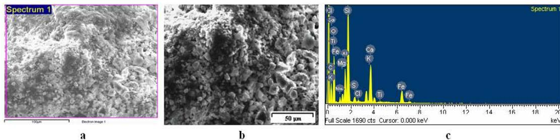
**Fig. 9.** SEM analysis for agglomeration of microscopic fine particles: a) and b) SEM images, and c) EDX spectrum [5].
