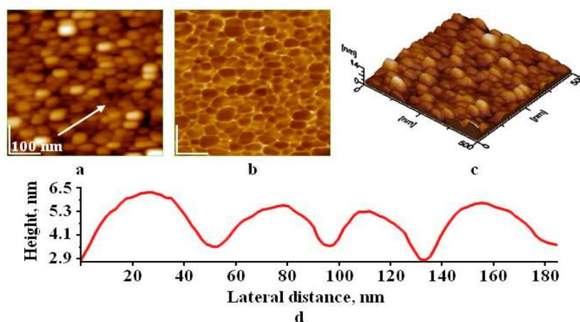
**Fig. 20.** AFM images for submicron particles from Aurel Vlaicu street; a) topographic image, b) phase image, c) 3D image of figure (a), and d) cross profile along the white arrow in the image (a). Scanned area: 500 nm x 500 nm [5, 91].
