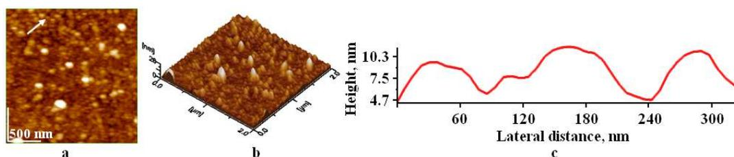
**Fig. 10.** AFM images of Aurel Vlaicu street dust sample, adsorbed on glass plate, optically polished: a) topographical image, b) 3D image of figure (a), and c) cross section along the white arrow in image (a). Scanned area:  $2 \mu\text{m} \times 2 \mu\text{m}$  [5, 91].
