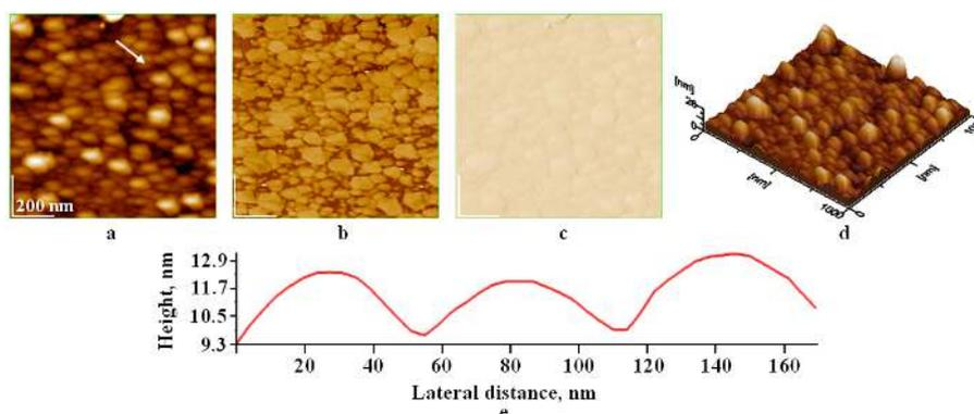
**Fig. 6.** AFM images of dust sample collected from Dâmboviței street, adsorbed on glass: a) topographical image, b) phase image, c) amplitude image, d) 3D image of figure (a) and e) cross profile along the white arrow in figure (a). Scanned area:  $1 \mu\text{m} \times 1 \mu\text{m}$  [5, 93].
