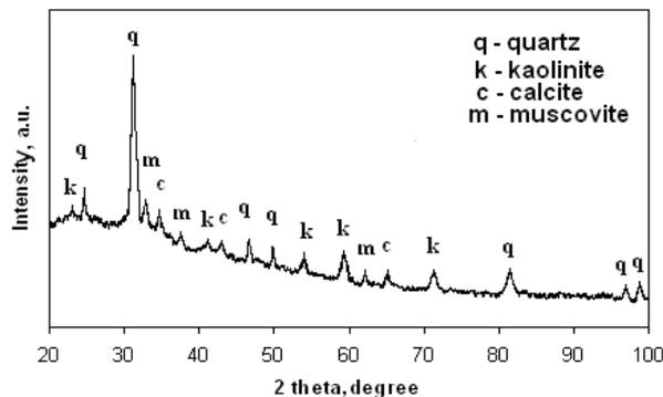
Fig. 1. XRD pattern for clay ground sample [5].
