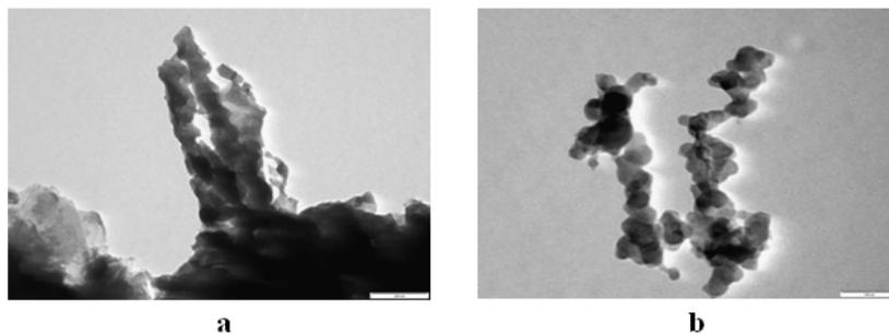
**Fig. 3.** TEM images proving street dust particles fragmentation until nanostructure level: a) clay and quartz submicron particles and b) clay nano-particles [5].
