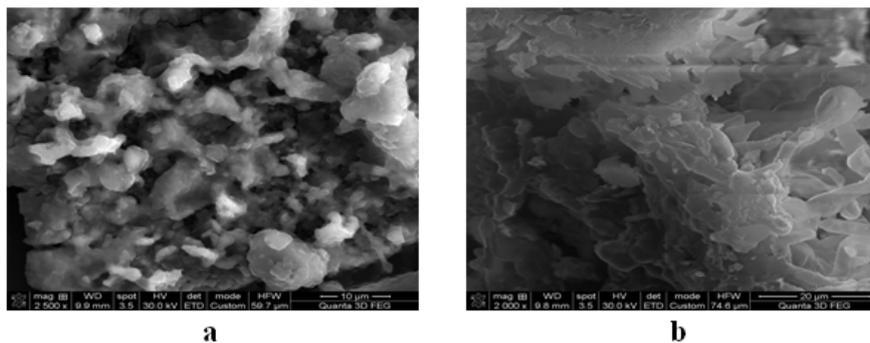
**Fig. 15.** SEM images of PM2.5 in powder material collected from air: a) Dâmboviței [5, 92] and b) Aurel Vlaicu streets [5].
