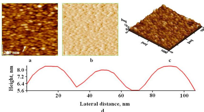
**Fig. 19.** AFM images for submicron particles from Dâmboviței street; a) topographic image, b) amplitude image, c) 3D image of figure (a), and d) cross profile along the white arrow in the image (a). Scanned area: 1000 nm x 1000 nm [5].
