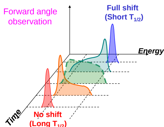
Fig. 1. Illustration of the DSA method for the lifetime measurements using the gamma-ray lineshape analysis.
