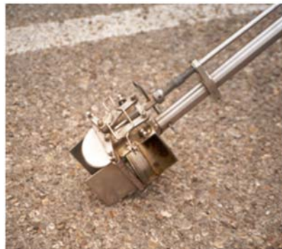
Fig. 2 - Sampler used to draw surficial sediments.
