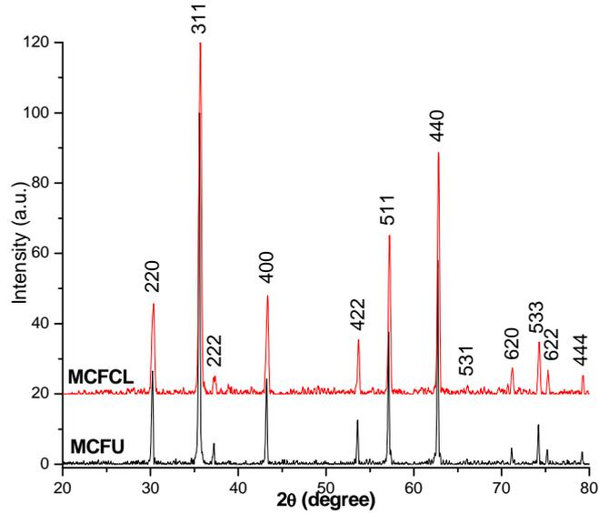
**Figure 3.** X-ray diffraction patterns of  $Mg_{0.5}Cu_{0.5}Fe_2O_4$  powders heated at 1073K
