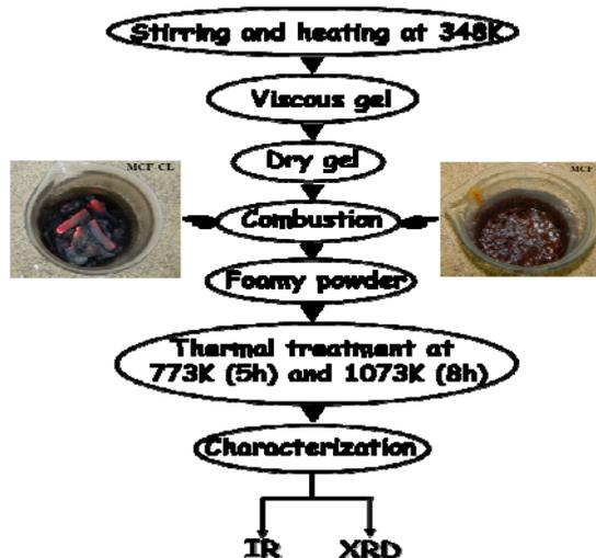
Figure 1. Flowchart of the powder preparation
