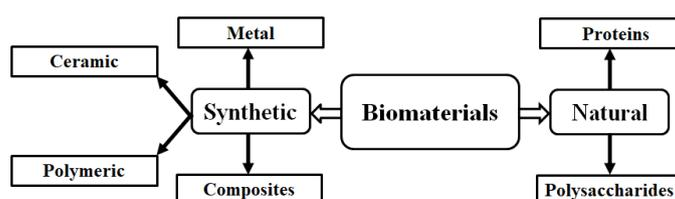
**Fig. 1.** Classification of biomaterials according to origin
